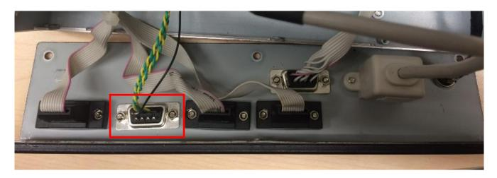
Step 6: Connect original COM1 cable to CN19.
