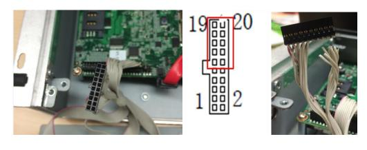
Step 4: Take 170002043 (COM2 cable) from accessory box, connect to M/B CN20.
