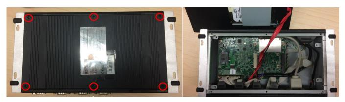
Step 2: Remove 3 screws on front panel and take off front panel. (Keep the cable on the front panel.)
