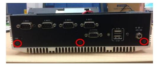
Step 3 : Disconnect the cable from M/B CN19, cut off cable 11~20pin as below picture. And remove the COM2 connector on front panel.
